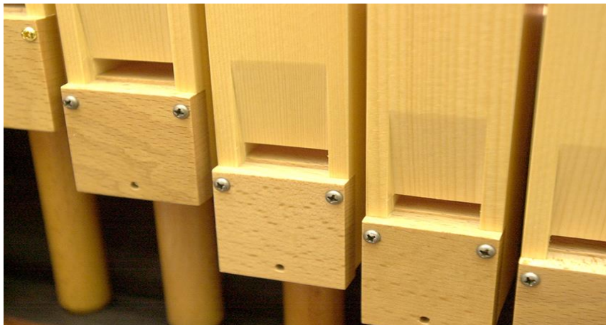
Wooden Pipes. These are made of four pieces of spruce wood glued together. Below is the rank of Wald Flute pipes
