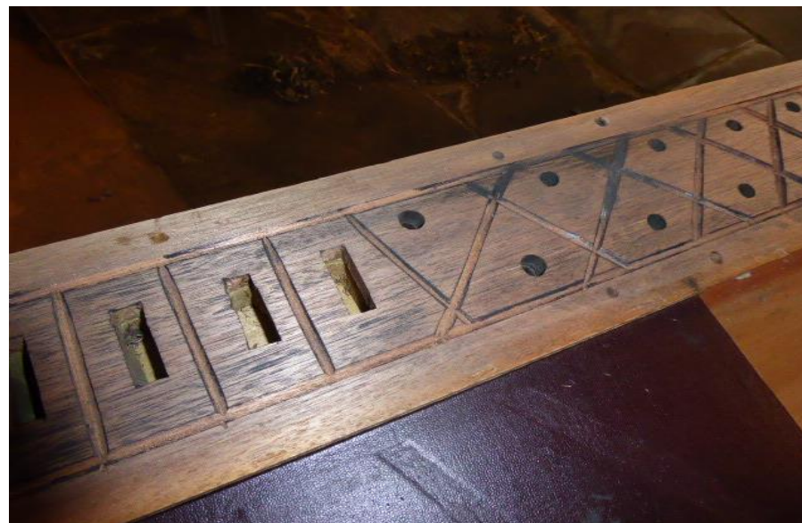
When a stop is pulled a long piece of wood called a slider opens up the holes for air into the pipes. The slider lies across the board shown above, called the “sound board”. The grooves prevent air leakage from one pipe to the next.
