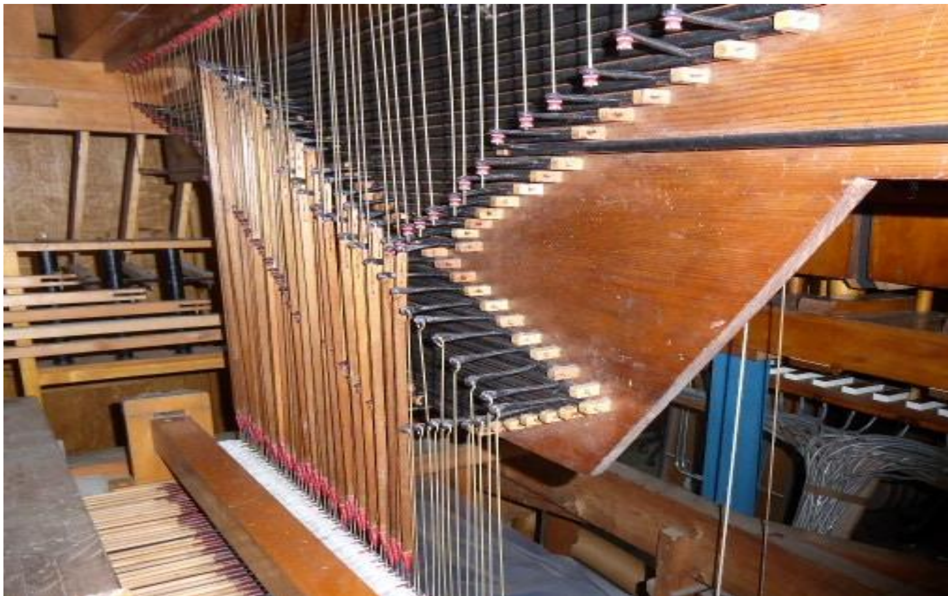
This is the swell roller board with the Bourdon pipe valves on the right and stop connections to the left.
